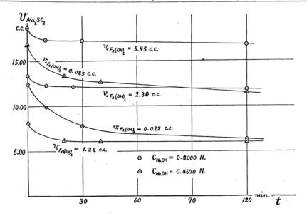
As is shown in Table 1 and 2, the oxidation velocity of sodium sulphite in the presence of ferrous hydroxide by means of air decreases rapidly with
